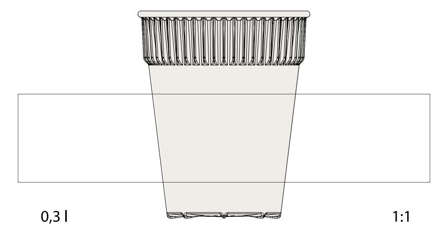
Outlines, lines, text or lettering printed on rotary screen print machines without the use of a backing colour with thickness under 1mm may result in reduced resistance to mechanical and chemical damage. For this reason, we recommend creating graphic documents with this minimum specified thickness for rotary screen printing.
